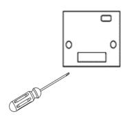
Remove the wired controller from the backing plate using a flat headed screwdriver in the gap between the backing plate and the controller. Once the two parts are separated, the remainder can be unclipped.
